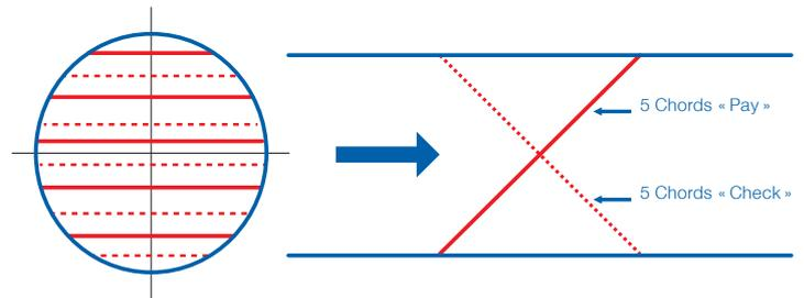
Performance and quality of measurement are improved by the addition of a 6th (or 11th) central path placed in the vertical plane; dedicated to the velocity of sound measurement as well as the detection of stream inhomogeneities such as gas, deposits, etc.
